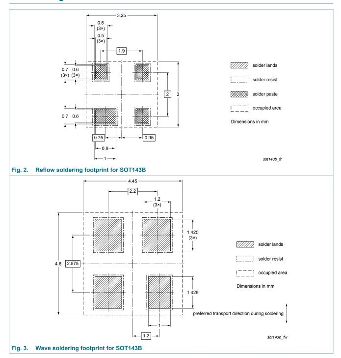
plastic, surface-mounted package; 4 leads; 1.9 mm pitch; 2.9 mm x 1.3 mm x 1 mm body
